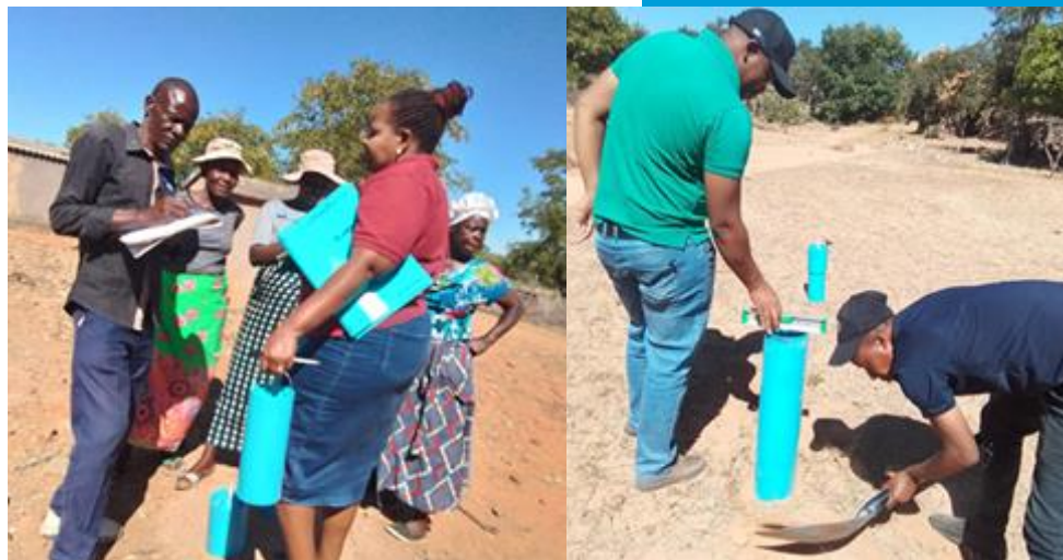
Mrs. Chirenje in maroon t-shirt on the left, training the locals, and Mr. Manyonga in green t-shirt making sure that the rain gauge is installed on a level platform.
