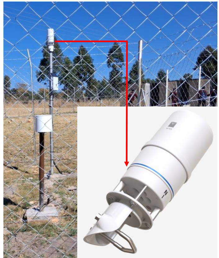
Ultrasonic Anemometer (right)
